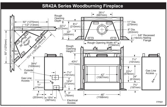
Fig. 3 SR42A Series specifications and framing.
